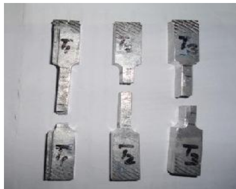
Figure 4. Tensile tested specimen (T1-3%, T2-6%, T3-12%)
